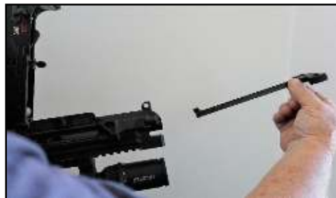
Remove the charging handle.
