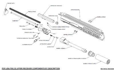
Now stand the bolt on the recoil spring guide rod retainer and apply downward pressure on the nose of the bolt (compress the spring) to remove tension on the spring retaining clip. Slide the retaining clip off of the recoil rod. This will allow you to remove the bolt and the recoil spring from the rod. You will also be able to separate the recoil rod from the guide rod retainer. Pay close attention to the direction the retainer holds the rod.
