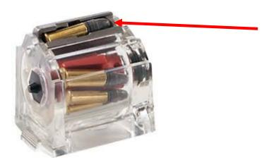
When rotor tension is correct the next round will be pushed up against the feed lips as depicted in this photo.
